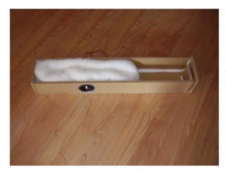
The stuffing is in the upper two third of the pipe and has a relatively high density.
