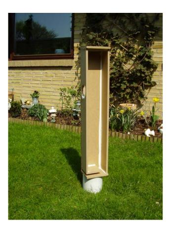
Even the opening is small; half the area of the driver Sd, there is no air turbulence (chuffing).
